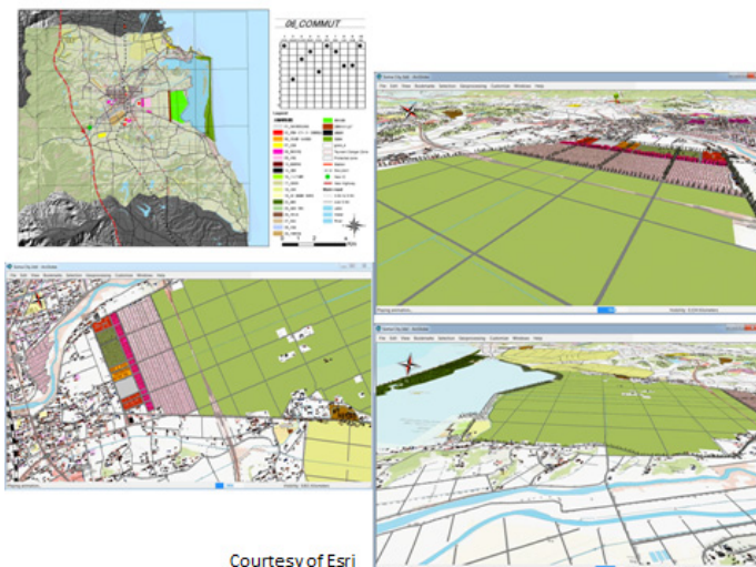
Fig. 12: From 2-dimensional GIS to 4-dimensional animation. Note that this design proposes to protect from future tsunamis by placing two manmade and forested barrier beaches surrounding a water park, and new agriculture and a raised bypass road between the new compact development and the ocean.
