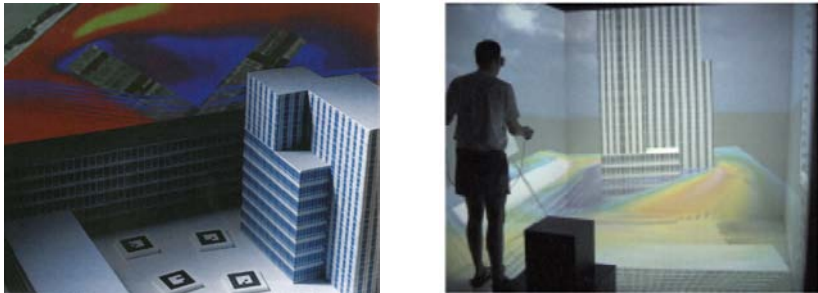
Fig. 4: Simulation of air flow in an urban skyscraper situation (right) configured on an interactive desk (left) (KIEFERLE & WÖSSNER 2003).
