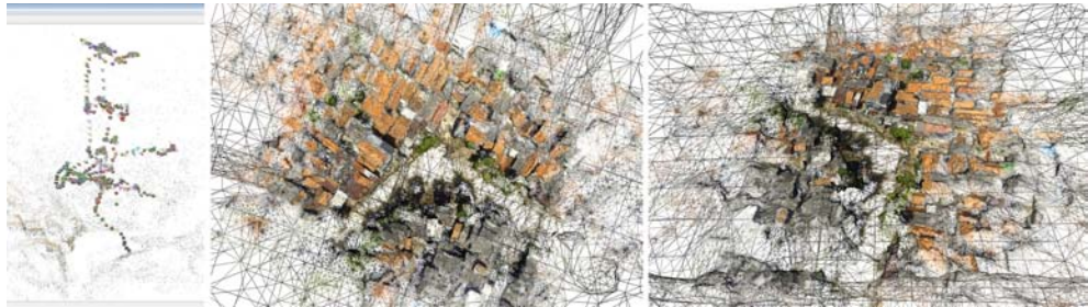
Fig. 11: Left: The Phantom copter produced overviews from specific height intervals, evident as three main levels (approx. 10, 20 and 30 m). Mid & Right: Overview (30 m altitude) site model, visualised in MeshLab.
