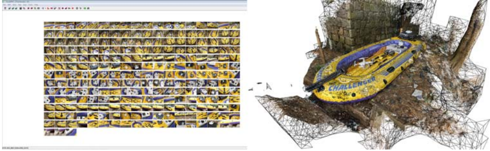
Fig. 6: Left: First step of the VisualSfM workflow – feature detection from a set of 237 photos as input. Right: Final textured surface model, generated in MeshLab.
