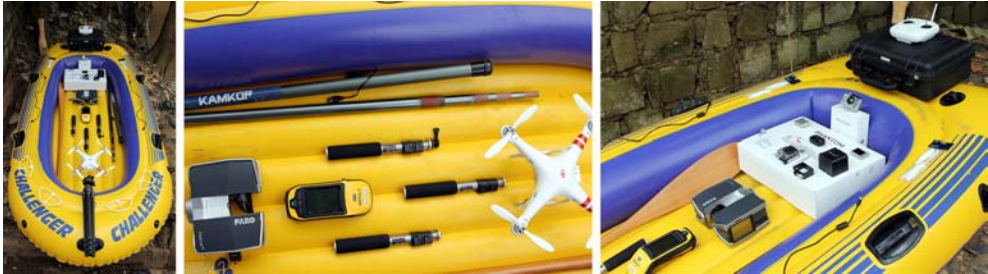
Fig. 3: Technological arsenal (2013). Visible are the GoPro action cameras, the DJI Phantom quadcopter, the FARO Focus3D high-speed 3D Laser Scanner and the TRIMBLE GeoXH Handheld Global Navigation Satellite System.
