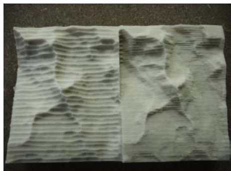
Fig. 2: Matterhorn, first tests: Different stepsize and precision (source: GEORGIOS ORFANOPOULOS)
